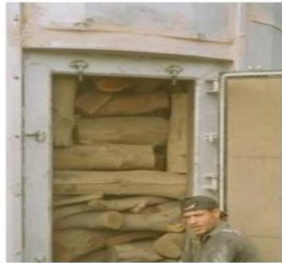
Mechanized charcoaling process with methane recovery
